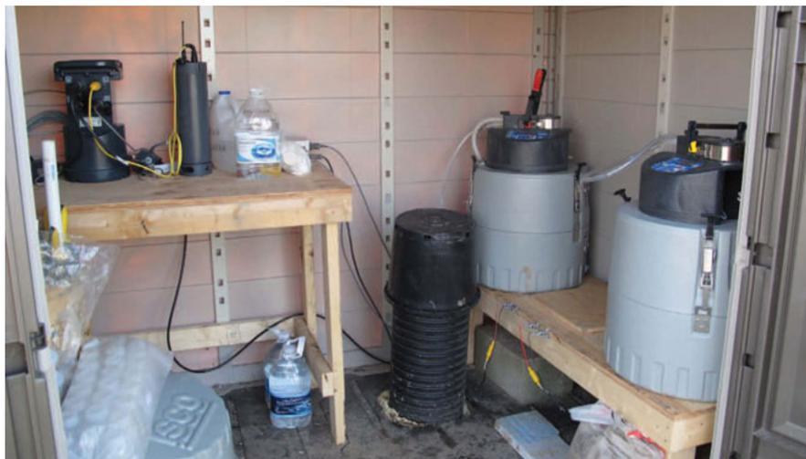
**Instrumentation used to monitor tile water flow and sampling collections on one of the farm field sites.**
